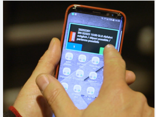
SBB conductors use a special widget placed on the home screen to signal engineers that the tracks are clear and the train is ready for departure.
